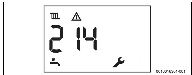
Fig. 12 Example of a fault code
